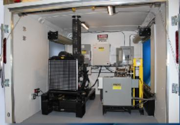
Roll up doors on the sides of the SAT allow instant access to the controls for the generator, as well as the compressor. This will allow for operation from outside of the SAT. Reducing time near the operational equipment and increasing safety.
